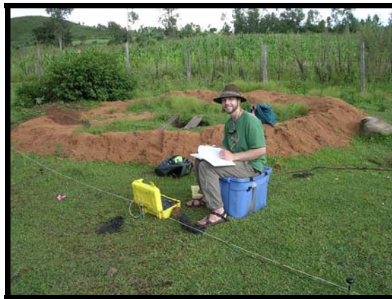
Figure 8 – Geophysical survey at one of the hand-dug well sites. Note the saprolite (well-weathered granite) material surrounding the well.
