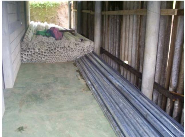
Both PVC and galvanized pipe were used in the system.
