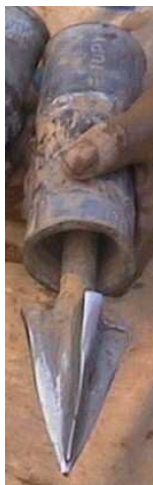
Drill Bit Welded at Local Shop
